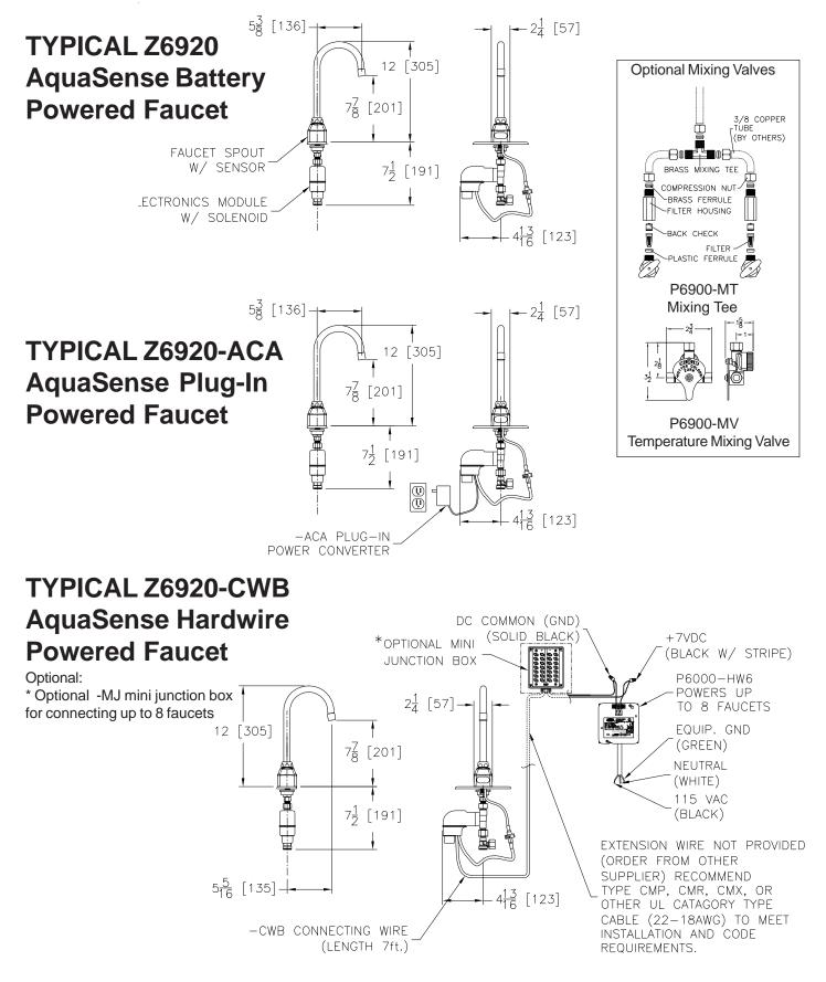
NOTE: MUST USE EITHER ZURN P6000-HW6 HARDWIRE POWER CONVERTER OR ZURN P6900-ACA PLUG-IN POWER CONVERTER TO ENSURE PROPER OPERATION. USING A POWER CONVERTER OTHER THAN ZURN MAY RESULT IN OPERATION MALFUNCTION OR UNIT FAILURE.
