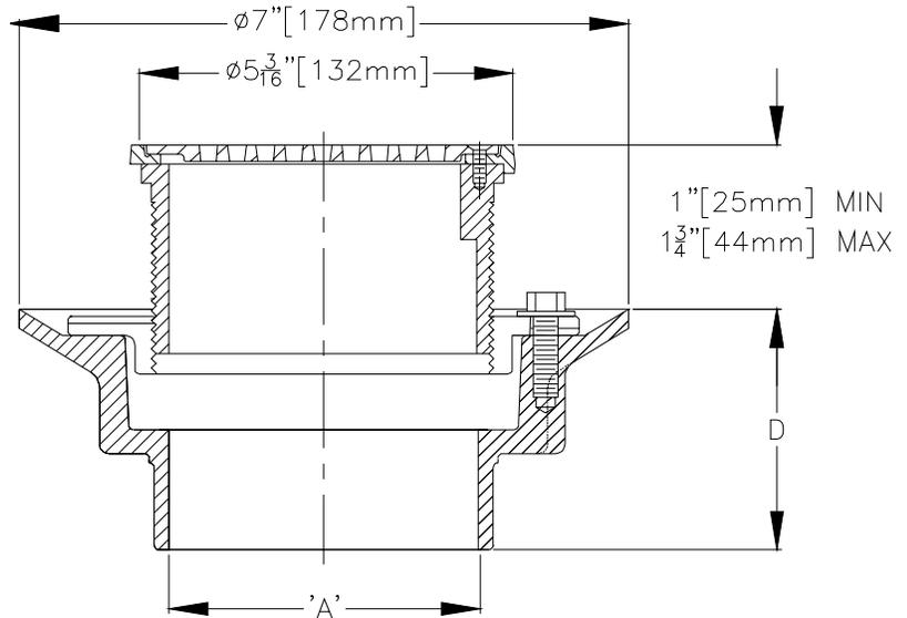
**FD-2321 Low Profile Adjustable Finished Area Floor Drain with Square Top**
