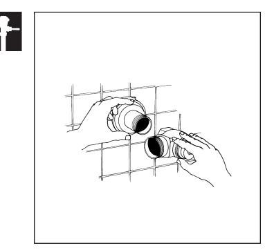
**1** Install stop valve using proper supply escutcheon and sweat solder kit if applicable.
