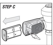
Sensor Adjustor Tool comes in a built-in storage pocket. Replace after use.
