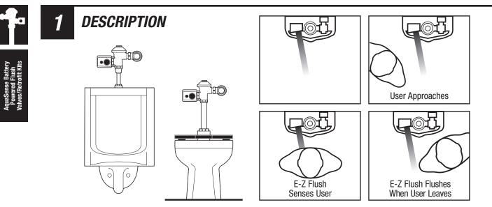
The E-Z Flush<sup>™</sup> sends out a continuous infrared beam that is reflected back by the presence of a person in front of the urinal or toilet. The technology differentiates between someone walking past the unit or actually using the fixture. E-Z Flush models ZERK-CP and ZERK-CPM retrofit Zurn and Sloan valves. For Delaney valves, order model ZERK-CP-LY or ZERK-CPM-LY.
