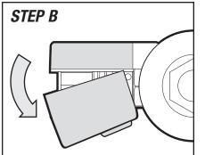
Pull cover off by rotating battery side forward and out.
