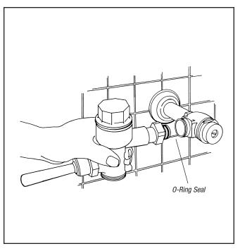
2 Insert flush valve tailpiece into stop valve, being certain 0-ring seal is in place. Wet seal with water to lubricate. Hand tighten locknut. Determine length of vacuum breaker tube required and cut as necessary. Assemble vacuum breaker tube assembly between flush valve and fixture spud.
