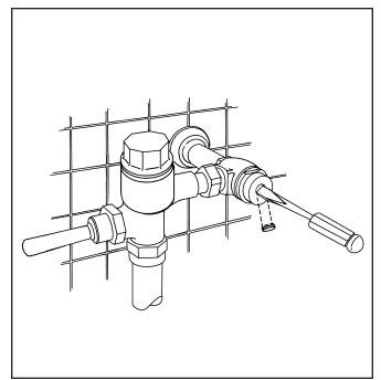
**4** Set flush valve for proper operation by adjusting stop valve. Stop valve adjustments can only be made by using the adjusting screw located behind the adjusting screw cover. (Water must be shut off at main supply valve if stop cap is to be removed.) Final setting should provide enough water flow to evacuate a closet fixture and should be such that a urinal fixture will not overflow when continually flushed. Secure adjusting screw cover.
