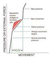
of the pocket at the maximum pressure or load, the wedge buttress are in shear. The maximum movement is about 0.3 inch through the thirty-six inch size and 0.4 inch for forty-two and forty-eight inch.
