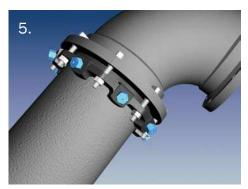
In large sizes (30-48 inch), five or more repetitions may be required. The use of a torque-indicating wrench will facilitate this procedure.
