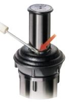
To adjust arc, depress pin and add to or subtract from existing arc, which as been preset to  $180^{\circ}$  at the factory.
