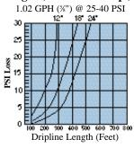
Friction Loss vs. Length of Run (Non-Pres.-Comp.)
