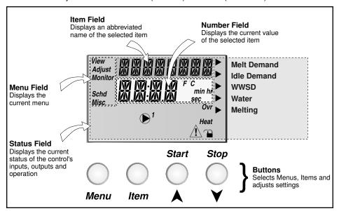
The tekmar Snow Detector & Melting Control 665 has a Liquid Crystal Display (LCD) and four push buttons (Menu, Item,  $\blacktriangle$ ,  $\blacktriangledown$ ) which are used to view and adjust the settings.
