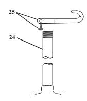
3. Screw no.23 down on no.24 and hand tighten, then tighten no.23 with a wrench, which will also tighten no.24. Make sure to align no.25 over center of sink, directly in front of no.24 while tightening.
