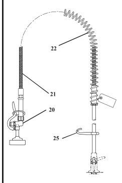
4. Adjust position of no.25 so that no.20 hangs loosely in it without straining no.21 or no.22.
