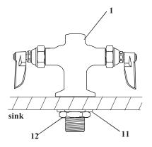
5. Install no.11 and no.12 on no.1, tighten no.12. Screw no.14 up on no.1, tightening by hand, *making sure to align pins on no*.13 *with corresponding holes at base of* no.1.
