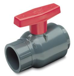
This heavy bodied, quarter-turn shut off valve is popular where maintenance-free installations are desired for a variety of chemical, industrial and OEM applications. Factory-adjusted sealed units are available in IPS sizes 1/2" through 6", with choice of socket, threaded or flanged end connectors.
