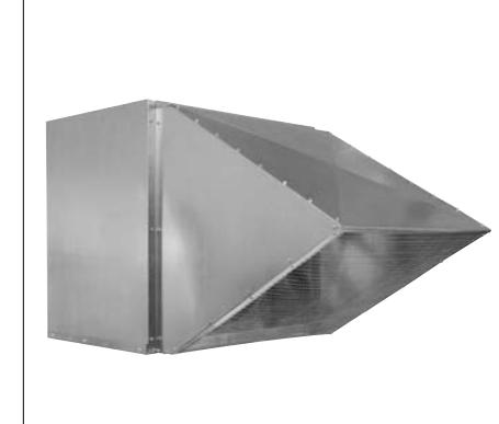
**Standard Duty Aluminum Supply Motorized Shutter:** The motorized option improves weather protection by providing a tighter closure seal and is recommended for all supply applications. Standard duty dampers are constructed with galvanized frames and aluminum blades and are rated to 2000 FPM. The damper body is not recessed providing extra clearance between the fan and damper blades. See page 19 for more details on the electric damper operators.
