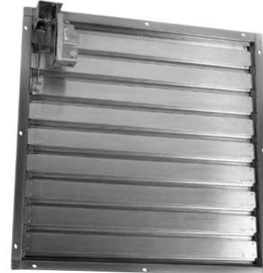
**Heavy-Duty Galvanized Exhaust Motorized Shutter:** This damper has a flanged frame and is designed to fit the inside flanges of the optional wall housing or wall mounting collar. The frame and blades are constructed of galvanized steel and are rated to 3000 FPM with proper clearance as provided by all factory accessories. The damper body recesses into the opening for a flush appearance. See page 19 for more details on the electric damper operators.
