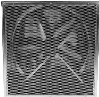
**Heavy-Duty Flat Wire Guard:** The removable safety guard satisfies OSHA requirements when used with the optional wall housing as a motorside (rear) guard. The H.D. expanded aluminum mesh is mounted in a galvanized frame and attaches to the inward flanges of the wall housing.
