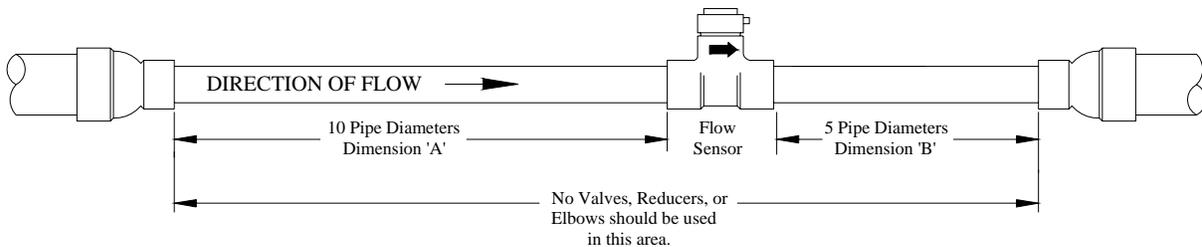
EXAMPLE: Using a 3 inch Flow Sensor:
