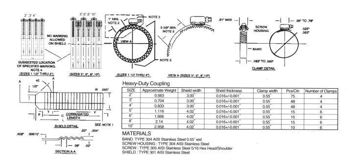
GASKET: Physical properties of gaskets complied with specification C564 EYELETS/RIVETS: TYPE 304 AISI Stainless Steel
