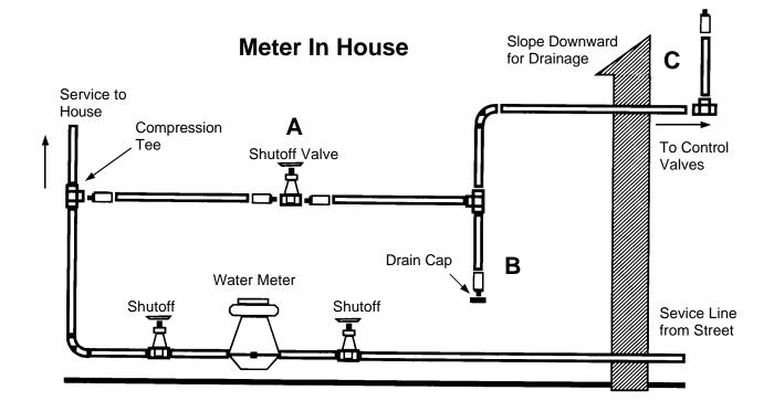
**Procedure: Wear proper eye protection.** The manual drain valve or drain cap is pressurized at this time and could cause physical injury if opened before the pressure is first relieved. Please follow the steps below carefully .
