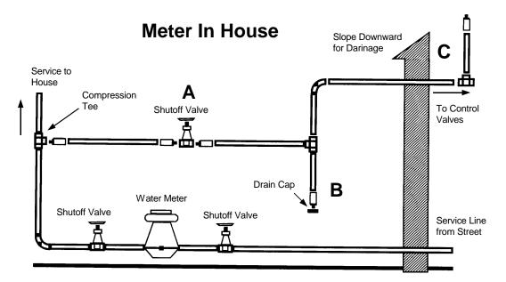
Procedure: Wear Proper Eye Protection! Do not stand over any irrigation components (pipe, valves, or sprinklers) during air blow out. Do not run the air compressor without a sprinkler zone control valve being open first, from start up to compressor shut down. Air pressure must not exceed 50 pounds per square inch (psi).
