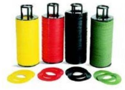
DF Series Disc Filter Rings. 80 Mesh (Yellow), 120 Mesh (Red), 140 Mesh (Black), 200 Mesh (Green)
