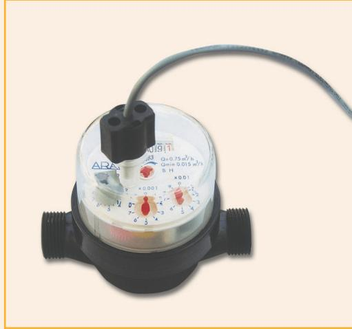
**Description:** The SF is a fertilizer and chemical solutions meter with electrical output and totalizing register. Inside the meter, the impeller is the only moving part that comes into contact with the liquid.
