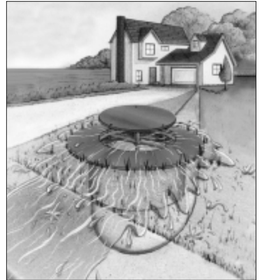
Allows water to flow to street without core drilling the curb.
