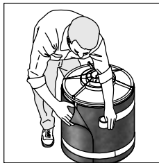
3 Optional Filter Fabric to prevent sand and debris from entering Flo-Well
