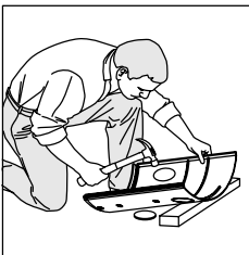
1 Knock out ports as needed from inside of panel
