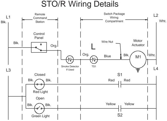
L3, L4 is a Supply Voltage Compatible with Lights and Switches. Standard Voltage is Same as Actuator Ordered.
