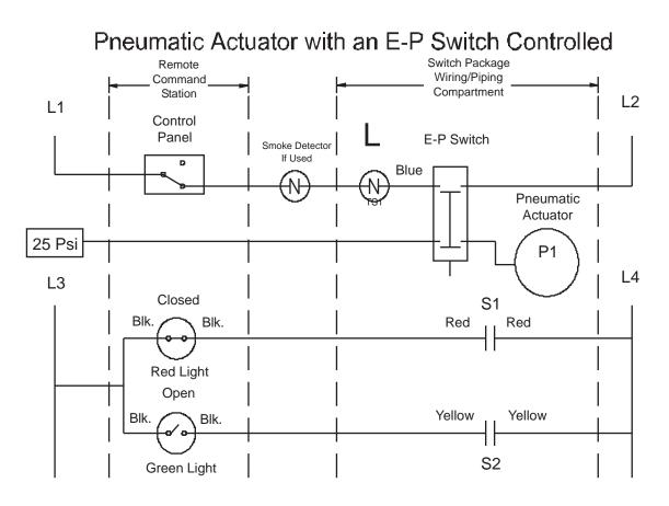
L1, L2 is the E-P Switch Supply Voltage desired (120vac or 24vac). L3, L4 is a Supply Voltage Compatible with Lights and Switches. Standard Voltage is 120vac if not Specified.
