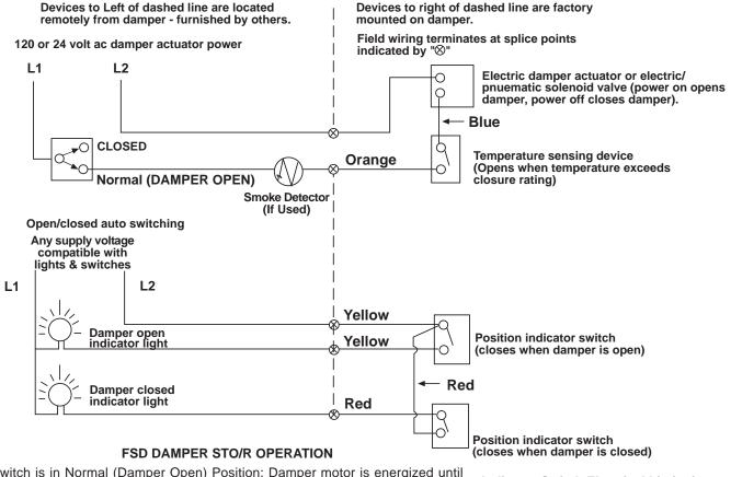
Switch is in Normal (Damper Open) Position: Damper motor is energized until thermostat senses temperature above initial closure rating. Above temperature closure rating, the damper motor is de-energized and damper closes.
