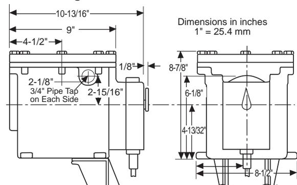
**Figure 5. Hazardous Location Housing Mounting Dimensions for Valve Actuators (See Valve Data for Valve Dimensions)**
