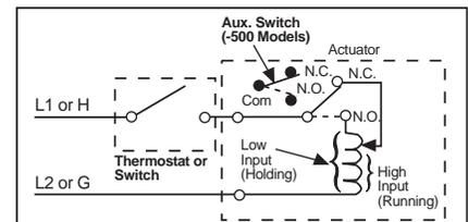
Figure 2. Wiring for MA-318, 416, 418 and 419 Series
