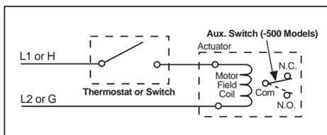
Figure 1. Wiring for MA-305 and 405 Series
