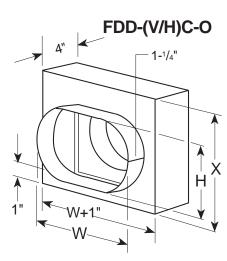
W = Width (Duct) H = Height (Duct X = Variable (See Size Chart)
