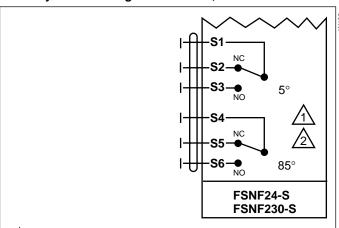
For end position indication, interlock control, fan startup, etc., FSNF24-S and FSNF230-S incorporate two built-in auxiliary switches: 2 x SPDT, 7A (2.5A inductive)@125/250 VAC, UL listed, 5° and 85°. Switch rating 250°F [121°C] 1/2 hour only.
