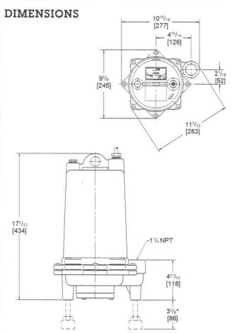
Leg kit required when not using guide rail liftout system.
