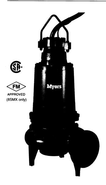
THE MYERS 8SM SUBMERSIBLE NON-CLOG SEWAGE PUMPS ARE DESIGNED ESPECIALLY FOR HIGH FLOW APPLICATIONS SUCH AS: large municipal lift stations, treatment plants, transfer stations and dewatering. A quick removal type rail system is available to simplify installation and maintenance. The 8SM's ability to handle solids up to 3 inches in diameter make it ideal for most high flow wastewater applications. For more information, contact your Myers distributor, or the Myers Ohio sales office at 419-289-1144.
