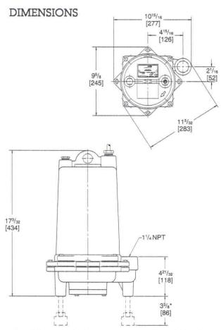
Leg kit required when not using guide rail liftout system.
