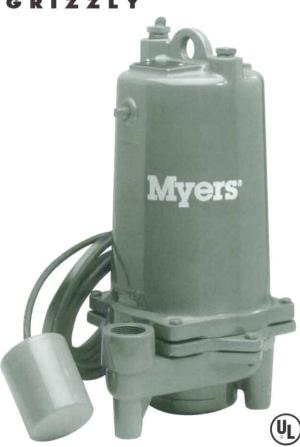
THE MG200 GRIZZLY™ IS A 2 HP SUBMERSIBLE GRINDER PUMP DESIGNED TO BE RUGGED AND ECONOMICAL FOR RESIDENTIAL AND PRESSURE SEWAGE APPLICATIONS. Long discharge runs or high static heads are not a problem. The Grizzly™ features a patented cutter mechanism and recessed impeller design to effectively macerate typical domestic sewage solids into a fine slurry.
