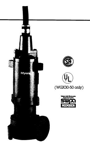
MYERS WG30-50 ARE RUGGED 3-5 HORSEPOWER SUB-MERSIBLE CENTRIFUGAL GRINDER PUMPS DESIGNED FOR RESIDENTIAL, LIGHT COMMERCIAL, INDUSTRIAL OR MUNICIPAL APPLICATIONS. They are especially designed for grinder pump applications requiring higher flows at low to moderate heads. The WG30-50 feature a heavyduty cutter mechanism and recessed impeller design to efficiently grind typical sewage solids into a fine slurry.
