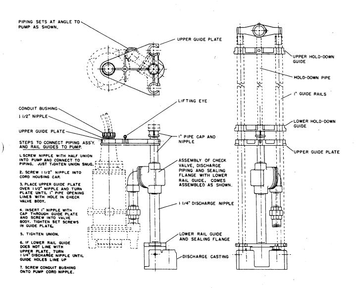
Do not install sealing compound into fitting until pumps have been run, to be sure all connections are correct.
