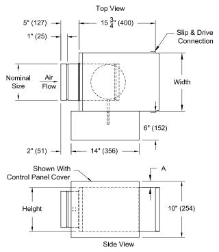
UNITS are manufactured with 20GA (1.0mm) Galvanized Steel Inlet Valve Assembly.
