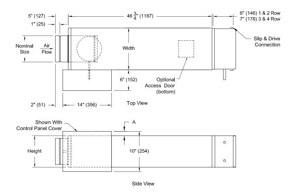
UNITS are manufactured with 20GA (1.0mm) Galvanized Steel Inlet Valve Assembly.
