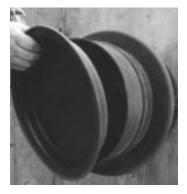
Place second end cap on sleeve. Check to determine that the cap is properly inserted.
