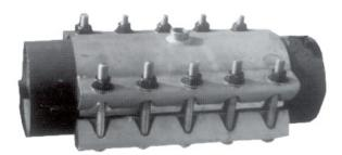
**Tapping Sleeve Bolting System -** with a triangular lug design, allows for pass-through, replaceable bolts. This lug configuration eliminates alignment problems and allows tightening from either side of the pipe.
