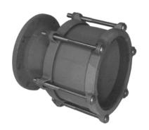
The JCM 306 Fabricated Flanged Coupling Adapter combine the versatile JCM Ductile Iron Coupling system with a fabricated flanged end to provide a fitting which allows for pipe misalignment, less critical pipe end preparation and ease of equipment installation and removal. The 306 FCAs are easily adapted from one type of pipe to another with the simple JCM Transition Gasket system. These FCAs simplify installations on larger A/C pipe and are available in the hard to find 10" and 12" sizes.
