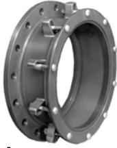
The JCM 303 Fabricated Flanged Coupling Adapter provides a simple means of joining plain end pipe to flanged fittings, valves and equipment. Fabricated from steel, these fittings are readily available in large or small sizes with a standard AWWA Class D flange. Special or heavier flanges are available on request.
