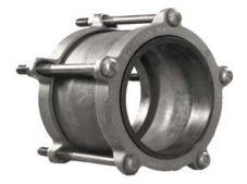
JCM Ductile Iron Couplings employ the mechanical compression joint principle to join two pieces of plain end pipe. This stress relieving flexible joint eliminates precise cutting and fitting in the field while providing for deflection, expansion-contraction, pipe settlement and a quick easy means of disassembling the system for maintenance.
