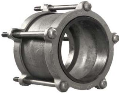
JCM Ductile Iron Couplings employ the mechanical compression joint principle to join two pieces of plain end pipe. This stress relieving flexible joint eliminates precise cutting and fitting in the field while providing for deflection, expansion-contraction, pipe settlement and a quick easy means of disassembling the system for maintenance.
