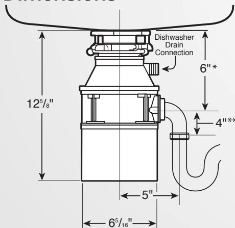
\* Distance from bottom of sink to center line of disposer outlet.
