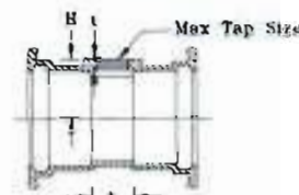
Service Tee. Gasket Joints on each end provide added degrees of freedom.
