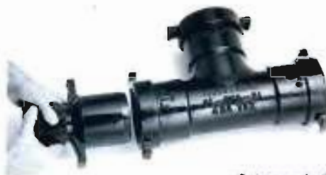
Spigot end of reducers insert into the bells of all other Harco fittings. Restraint rings "lock" reducers to main fitting. Patent Pending.
