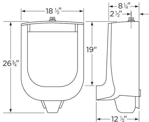
RECOMMENDED STATIC WATER PRESSURE FOR PLUMBING FIXTURES IS 20 - 80 PSI STATIC PER ANSI STANDARDS A112.19.2M APPENDIX B.
