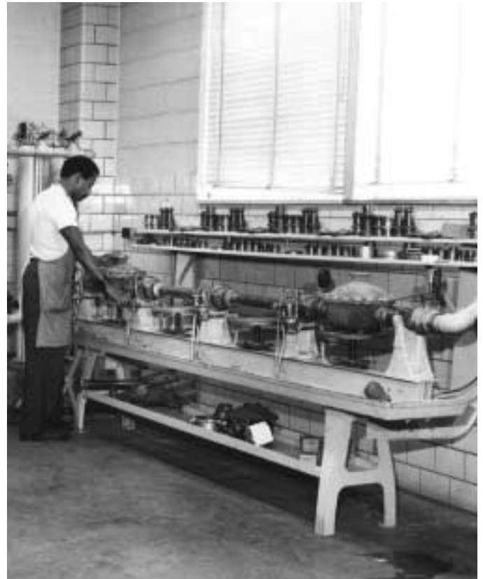
The No.4 Akron Bench is used for testing 1-1/2" and 2" meters. The machine includes a Double Range Testerate Indicator and test tanks.
