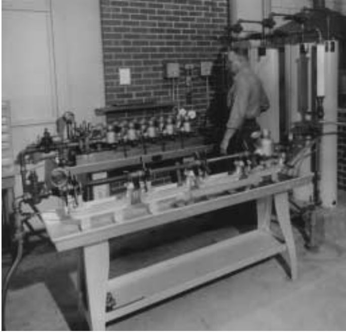
This meter shop has a No. 4 Standard Test Bench with Testerate Indicator and Electric Flow Control Valve, Nos. 1-F and 10-FG Calibrated Tanks. The bench is adapted to test 1-1/2" and 2" meters by a Tester Clamp.
