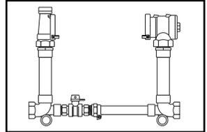
ANGLE KEY VALVE BY ANGLE DUAL CHECK VALVE (2" METER)
