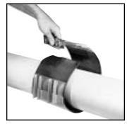
Back off nuts to end of bolts, but DO NOT remove them. Separate clamp and wrap it around the pipe by holding the lifter bar and bolts above the pipe and sliding the receiver section under the pipe.
