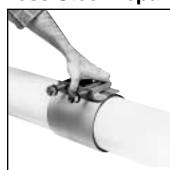
Slide the lifter bar up the receiver lugs and snap into place. Spin one of the nuts hand tight.
