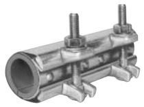
Ford Wrap Clamps offer the same Leak Repair features of the Snap Clamp with the extra assurance of 360° gasket coverage. Specific sizes are available for I.P.S. steel or copper. The All Stainless Steel Wrap Clamp offers the same conveniences and performance of the traditional Wrap Clamp with the added security of stainless steel lugs and bolts.
