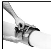
Bring the lifter bar and receiver section together at a convenient position on top of the pipe.
