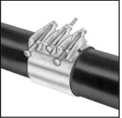
ROTATE THE CLAMP in the direction of the arrow.
