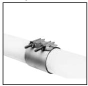
Tighten all nuts evenly with a balanced torque of 75 ft lbs or as tight as possible with a 12 inch wrench.
