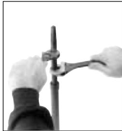
3. Insert the Boring Bar (DMBB) into the body of the machine until the shoulder hits the stop. Gently tighten the Packing Bushing (DMPB).
