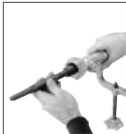
4. Select the Adapter (DMA) that matches the outlet threads on the corporation stop. Attach the Adapter (DMA) to the bottom of the Drilling Machine.
