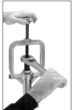
8. Slowly reverse the Feedscrew (DMHF) and allow the Boring Bar (DMBB) to back out until it hits the top stop in the machine. Close the corporation stop and release the entrapped pressure before removing the Drilling Machine from the corporation stop.
