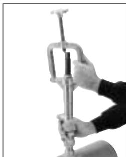
6. Carefully lower the Drill (DMD) until it touches the water main. Attach the Ratchet (DMRW) to the top of the Boring Bar (DMBB). Raise the Yoke (DMY) until the Feedscrew (DMHF) is centered over the Boring Bar (DMBB). Place a few drops of oil on the point of the Feedscrew (DMHF) and mate the point with the center of the Boring Bar (DMBB). Open Chip Flushing Port (if equipped.)
