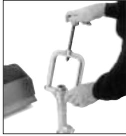
2. Select the diameter of Boring Bar (DMBB) which will pass through the corporation stop when it is open. Attach the Drill (DMD) to the Boring Bar (DMBB) and lightly tighten with the adjustable wrenches.
