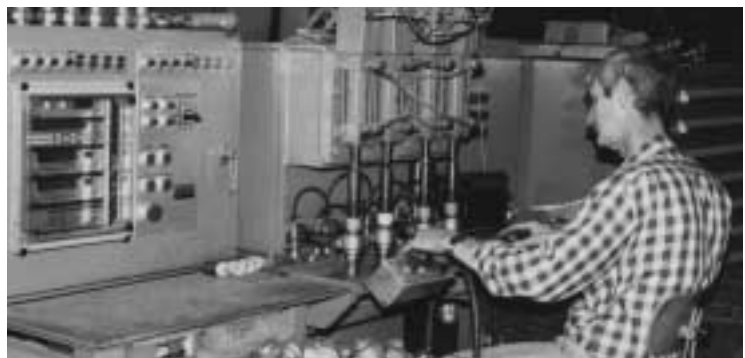
Ford check valves are tested on an environmentally safe "air-decay" tester.
