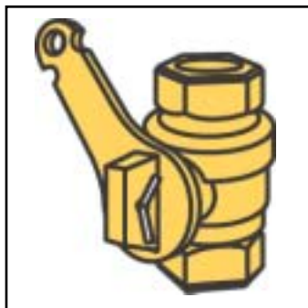
HP-4 for use on Ball Valves for Pitometer service
