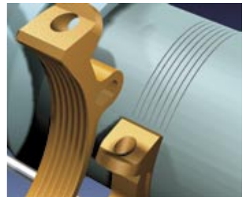
Image depicts Impression of Restraint on PVC pipe.
