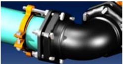
3. Using the connecting bolts to determine the proper restraint location, install both halves of the restraint by tapping them into place. Allow enough room on connecting bolts to fully engage the nuts. Make sure the complete ID of the restraint is touching the pipe before installing and tightening of side bolts. Side bolts are to be evenly tightened to 110 ft - lbs of torque (60 ft - lbs on 4" and 6").
