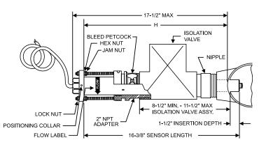
NOTE: ALL DIMENSIONS ARE FOR REFERENCE ONLY. TO REMOVE THE FLOW SENSOR THERE MUST BE 35" OF CLEARANCE ABOVE THE OUTSIDE WALL OF THE PIPE. A CUTTING TOOL MAY REQUIRE ADDITIONAL CLEARANCE.
