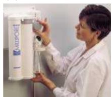
As long as the green LED is on, the water quality is above 1  $M\Omega$ ·cm at 25°C. When the LED is red, it's time to change the purification pack (DI-PAK) $^{\text{\tiny TL}}$ .
