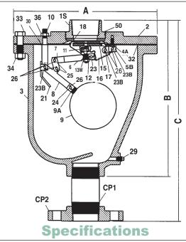
The valve(s) shall be installed at the high points in the system or at points selected by the engineer. This will permit discharging the surge of air from an empty line when filling, and relieve the vacuum when draining the system. The valve(s) shall also release an accumulation of air when the system is under pressure. This shall be accomplished in a single valve body.
