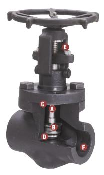
RP&C forged steel globe valves are designed and manufactured for extended service life under severe temperature and pressure conditions common to refinery, chemical and processing applications. Available in sizes from 1/2" to 2", these valves are designed with an integral CoCr-A body seat. CoCr-A seat rings are brazed into the valve body.
