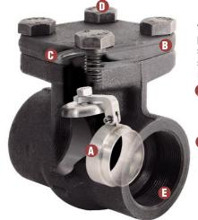
Innovative swing check design allows for full opening and highest Cv values possible, from 5.1 to 91.6. Available in sizes 1/4" to 2", standard 316 stainless steel swing unit and B7M bolting meets requirements of NACE MR 01-75.
