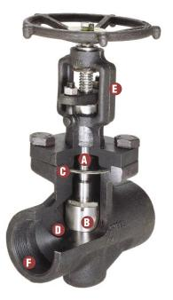
RP&C forged steel globe valves are designed and manufactured for extended service life under severe temperature and pressure conditions common to refinery, chemical and processing applications. Available in sizes from 1/4" to 2", these valves are designed with an integral CoCr-A body seat. CoCr-A seat rings are brazed into the valve body. Our globe valves use a Type 420 HT&H (500 Brinell) stainless steel disc.
