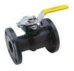
**88A-100 Series**—Carbon Steel Class 150 Flanged, Regular Port Valves. Unibody to 2", easily-repaired split body 2-1/2" and larger. (88B series is unibody design 3" and 4"). Standard stem grounding and locking device. Includes ISO 5211 mounting pad. Meets all standards, including NACE when ordered with SS trim, and API 607 4th Ed, when ordered as -24. Available in 1-1/2"-10".
